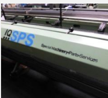
IQ-SPS projectile weaving machine, 7m weaving width
